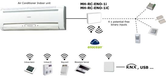
IntesisBox<sup>®</sup> MH-RC-ENO-1i allows monitoring and control, fully bi-directionally, all the functioning parameters of MITSUBISHI HEAVY INDUSTRIES Air Conditioners from EnOcean installations.
